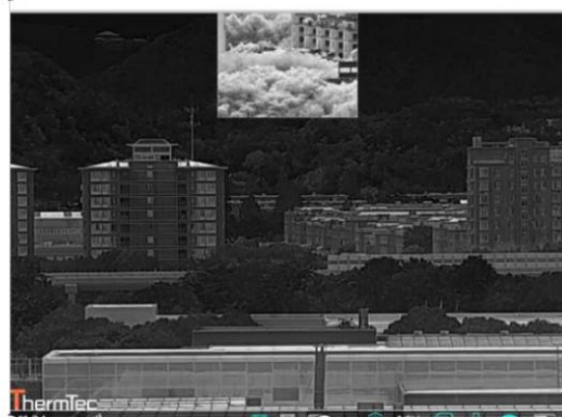
Main screen:Thermal imaging PIP:White Light/Night Vision
